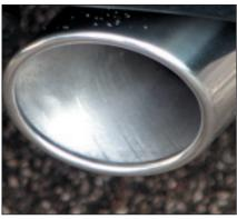
Although the tailpipes on this particular car were similar to those used by Jaguar, Elite will have a choice of three types, the one shown which is adjustable, slightly larger and fits the earlier bumper style XK8s well, a much larger oval type and a twin tailpipe system like that on the latest XKR.
