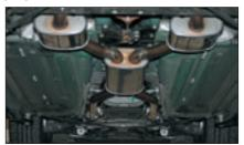
The centre silencers have a balance pipe built in, this eliminates any possibility of horrible noises from back-draft emitting from the pipes on the over-run.
