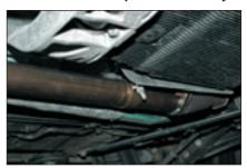
Aft of the catalytic converters, with the new system there are two new shortly stainless pipes. This provides an added benefit for those who want to extract even more performance from their XK. The removal of these two short pipes would allow the existing catalytic converters to be removed and replaced with an upgraded one for performance purposes.
