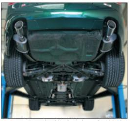
The underside of Mike's car fitted with the prototype Elite exhaust system, a good fit and finish assured.
